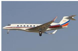
The Gulfstream G650 (yeah, like the singer who says, "..fly like a G6.."), has an Aspect Ratio of 7.7. If the wing area (S) is 1,283 ft², *determine the G650's wingspan (b)*.
